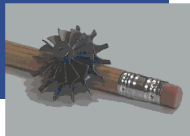
DARPA-Funded Microturbine Alternator for Portable Remote Electric Power
