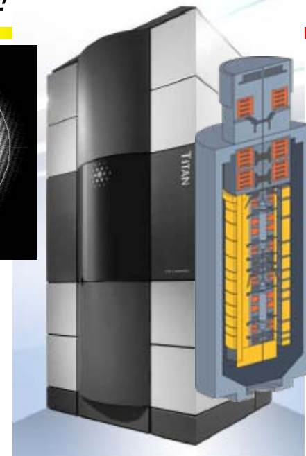
FEI Titan AC TEM/STEM for nanoscopy with the atomic resolution and sensitivity
